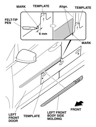
7. Align the left front body side molding with the mark on the template, and attach it to the left front door as shown.
