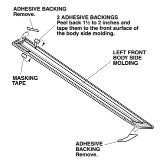
If the vehicle is equipped with accessory door edge guards, go to step 6. If not, continue with step 5.
